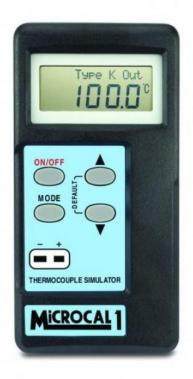
Thermocouple type K - range -200 to 1372°C
