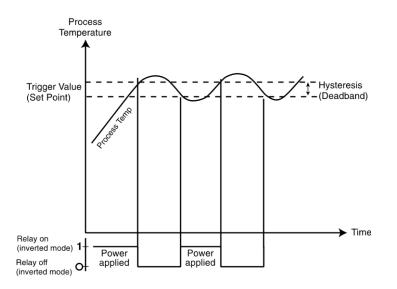
With On-Off temperature control, the output from the instrument is either on or off; the output is switched from one state to the other when the process temperature goes above or below the set point (trigger value). For the control of heating, the output is 'on' when the temperature is below the trigger value and 'off' when it is above the trigger value.
