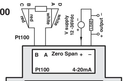
**Note 1:** The transmitter can be easily ranged and calibrated by means of the multi-turn zero and span adjusters in conjunction with either a mV source or standard resistance input.
