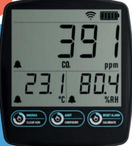
The EL-IOT-CO2 continuously monitors air quality and comfort levels, including CO<sub>2</sub>, a key indicator of adequate ventilation. It automatically uploads data to the EasyLog Cloud, allowing your complete set of data measurements to be viewed, analysed and downloaded from any internet-enabled device.
