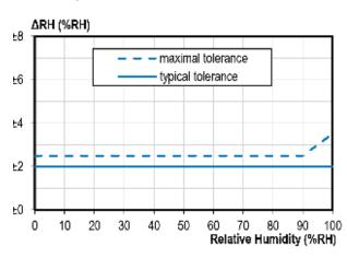
Typical tolerance of RH over Temperature:
