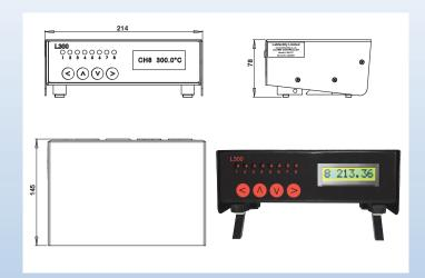
User interface Front panel keys for selecting channel
