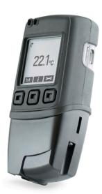
This standalone data logger measures and stores more than 250,000 temperature readings from a K, J or T-type thermocouple at a resolution of  $0.1^{\circ}$ C ( $0.2^{\circ}$ F). It comes supplied with a K-type thermocouple capable of measuring from 0 to 200°C (32 to 392°F).
